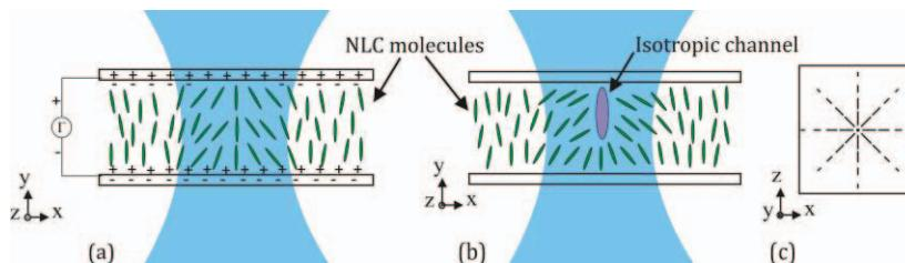
Fig. 1. Schematic distribution of the NLC molecule orientation (a) in the case of photorefractive effect and (b) in the case of isotropic channel formation in dye doped NLC; (c) the NLC director projection on the plane ZX.
