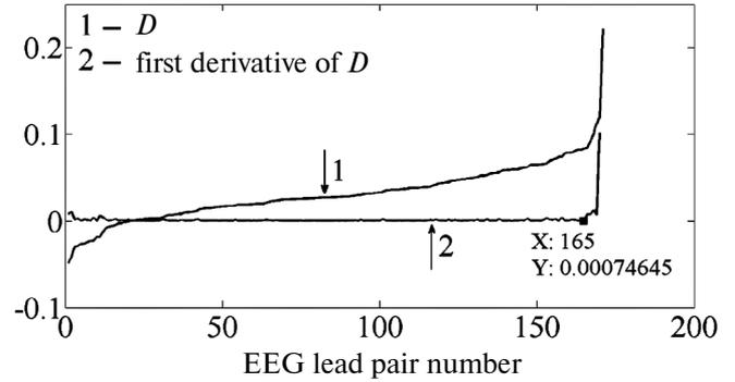
**Fig. 3.** 1) Curve of  $D$  vs. EEG lead pair number in the ascending order of  $D$ ; 2) first-derivative curve. The EEG was measured in a healthy subject.
