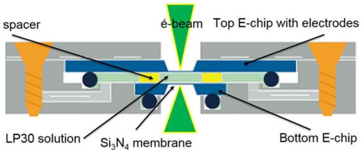
Figure1: Schematic presentation of sealed liquid cell
